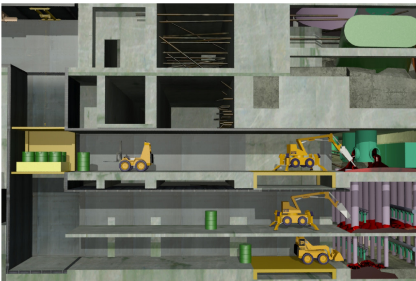
Fig. 6.27 — Access paths to fuel containing materials accumulations
