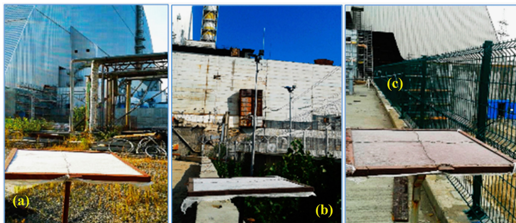
Fig. 4.8 — Deposition planchets in the Chernobyl NPP local zone: a — the north-western corner; b — the south-western corner; c — in the east
