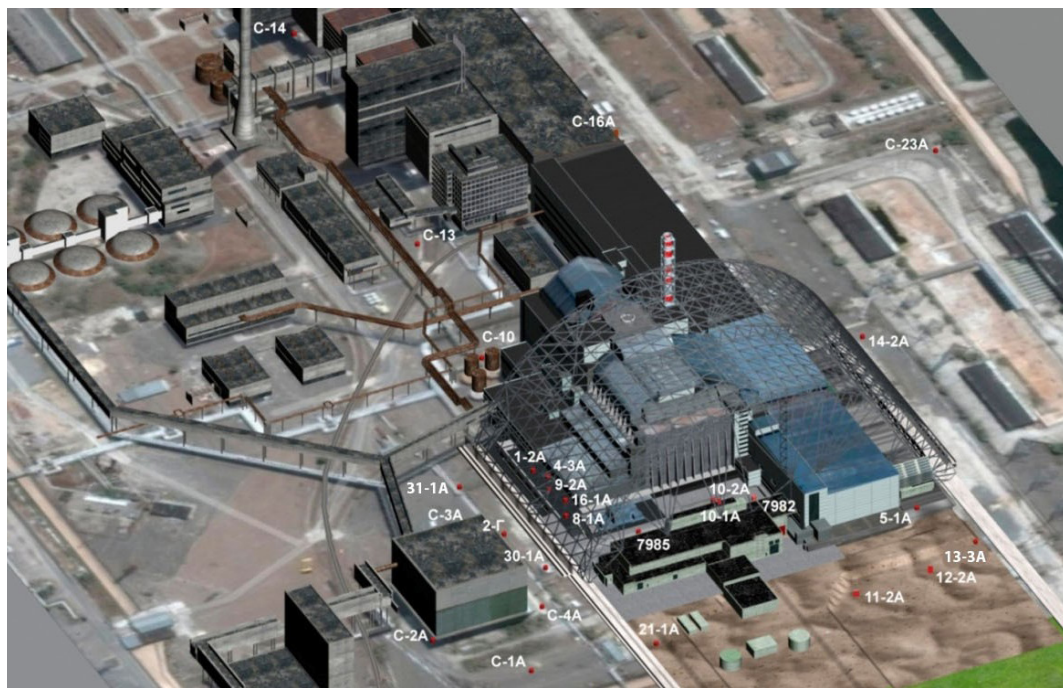
Fig. 4.10 — Location of radiohydroecological monitoring wells at the NSC area [138]
