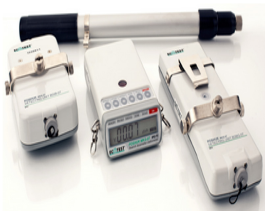
Fig. 3.1 — Radiometer-dosimeter MKS-07 “Poshuk” with the detection unit BDBG-07
